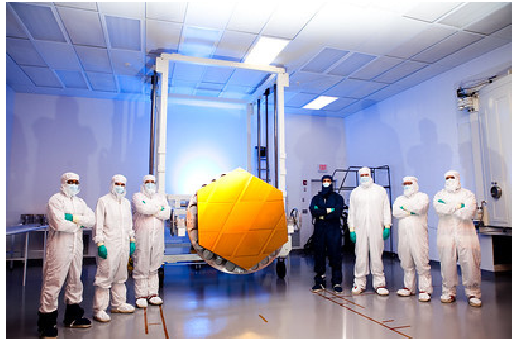
"Gold-coated Engineering Design Unit (EDU) Primary Mirror Segment" by James Webb Space Telescope is licensed under CC BY 2.0.
